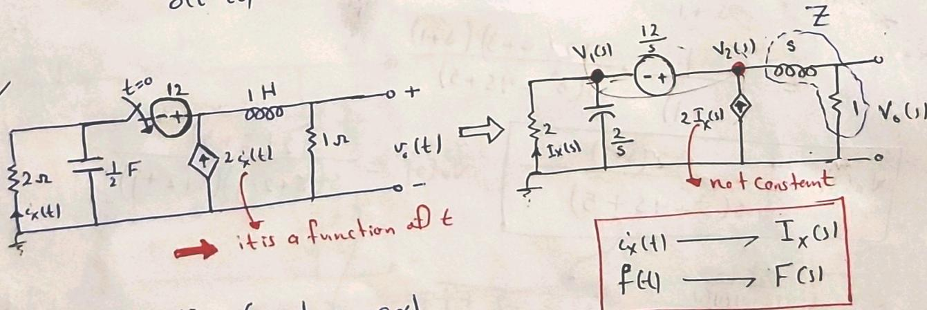
$v_2(s) - v_1(s) = \frac{12}{s}$  (constrain eq)
