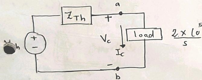
$$I_c = \frac{V_{TH}}{Z_{TH} + Z_{load}} = \frac{6s}{(s + 5000)^2}$$
